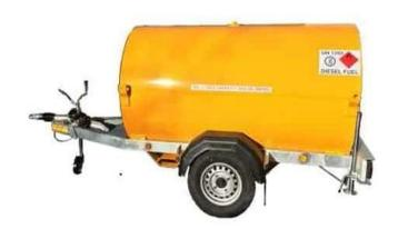
**AXLE/SUSPENSION:** Single Knott-Avonride 1500kg torsion beam axle fitted with 200 x 50 Auto reverse brakes.
