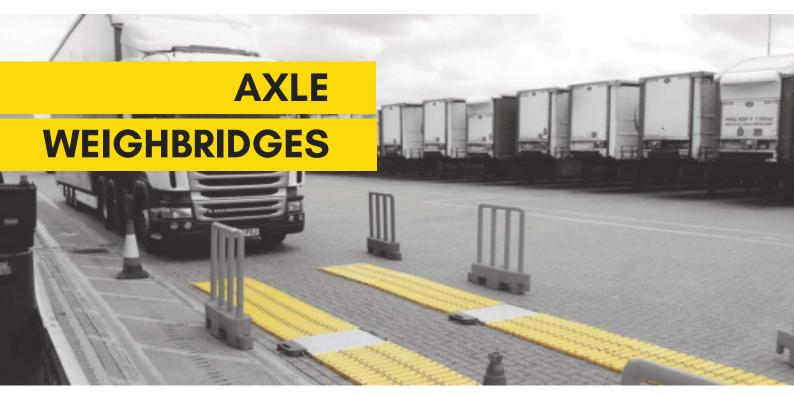
Vehicle Weighing Solutions offers a range of axle weighbridge solutions including high accuracy static weigh pads, fixed weighbridges and portable weighing in motion systems. Each of the systems are robust and offer high accuracy weighing.
