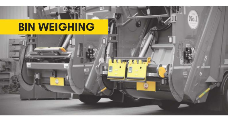
ENVIROWEIGH is a trade certifiable dynamic bin weighing system - accurate to class Y (b). It can be installed onto most types of RCVs lifting hoists and weighs the precise weight of waste collected from wheeled bin containers during the normal loading cycle. There is no need to stop the lifter and speeds are not compromised. Each lifting chair is installed with a weighing load cell and can weigh two bins independently and simultaneously.
