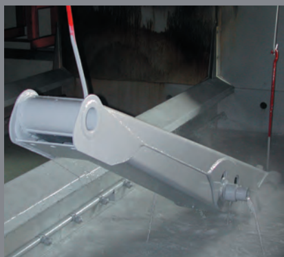
KTL-coating with burn-in process at 160°C
