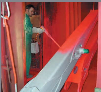
Powder coating with burn-in process at 200°C
