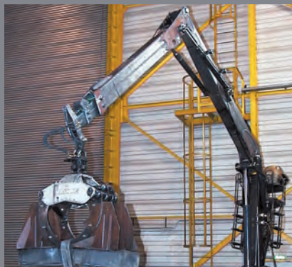
Endurance test on modern test benches by full capacity utilization
