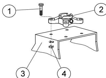
Insert the drive shaft on the rotator into the adapter (2) and secure it. (See the rotator manual for details).
