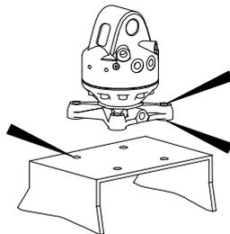
Position the adapter (2) (see Fig., Page 8 above) on the bucket carrier (3), and attached it with four screws (1) M16 (property class min. 8.8), washers and new locknuts.
