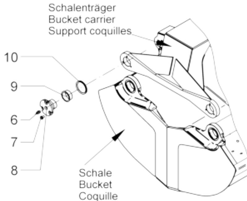
Screw the threaded rod of the falling weight device into the thread M16 of the main bearing pin. The main bearing pins can be pulled out by powerful dashes of the falling weight in the direction of arrow.
