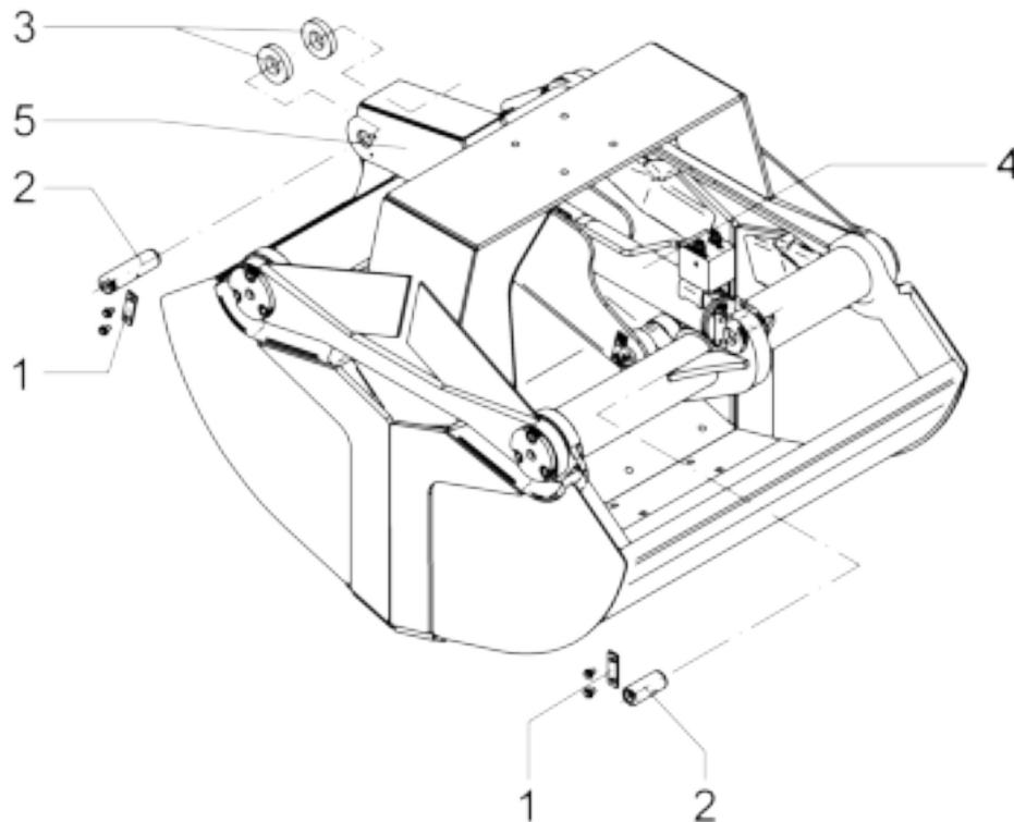
Remove the axle holders (1) and drift out the pin (2) .
