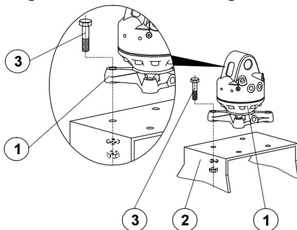
Position the rotator KM04 / KM 06 (1) on the bucket carrier (2), and attach it with four screws (3) M16 (property class min. 8.8), washers and new locknuts.
