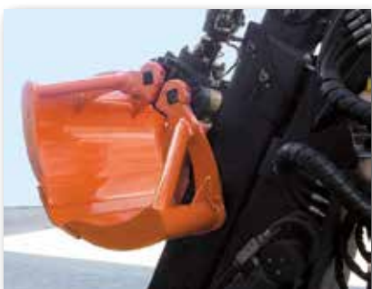
Universal Grapple for Z-Cranes KM 605U HPX-Z
