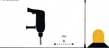
Drill hole in cab roof 12mm
