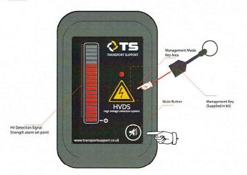
3.2 The HVDS will enter set-up mode and display the current alarm limit on the signal strength meter. By pressing the mute button the alarm limit can be incremented one LED bar at a time. Once the limit reaches the top of the display it will automatically drop back down to the bottom.
