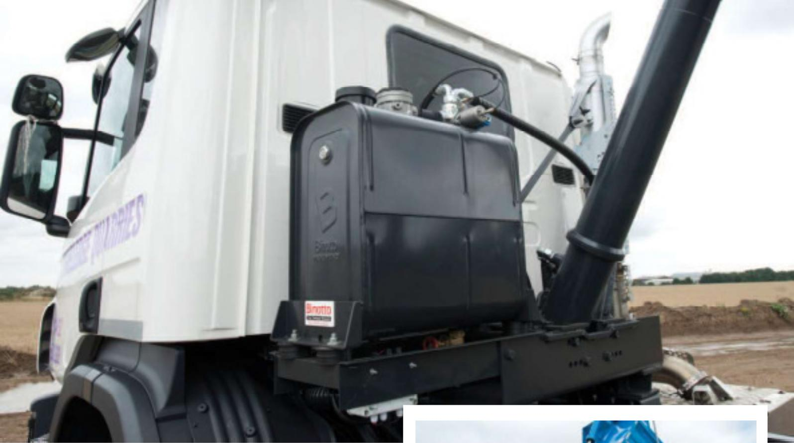
Binotto MFC Front End Tipping Gears are a separate cylinder and oil tank designed system for rigid vehicles from 7.5 to 36 tonnes G.V.W.
