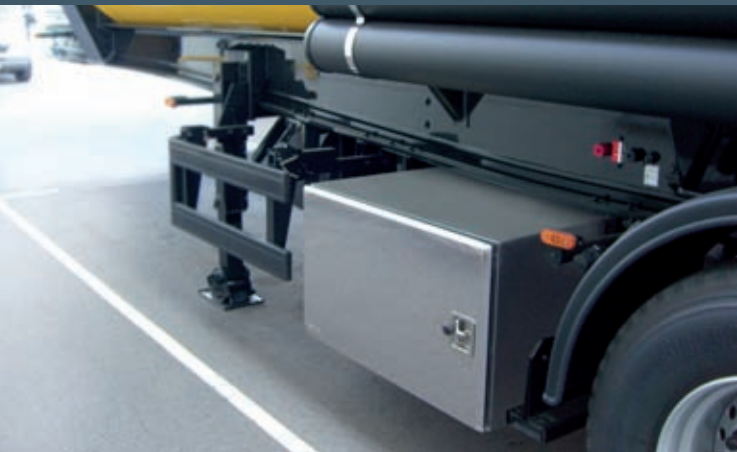
Fitting-out with BAWER 36 MONO toolbox with lateral opening.
