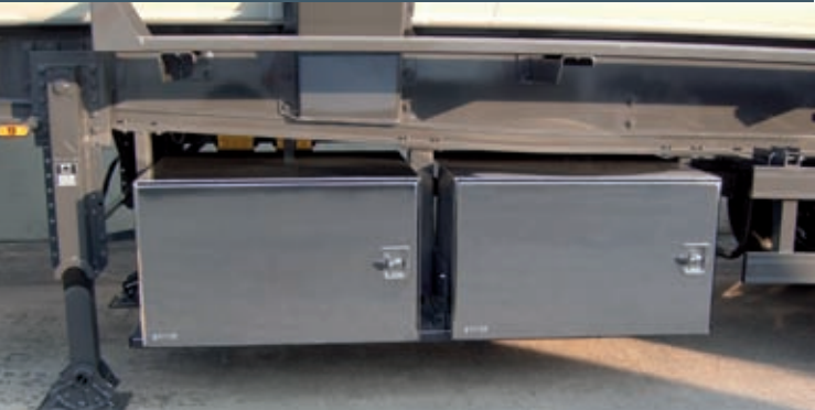
Fitting-out with two BAWER 37 MONO toolboxes with lateral opening.
