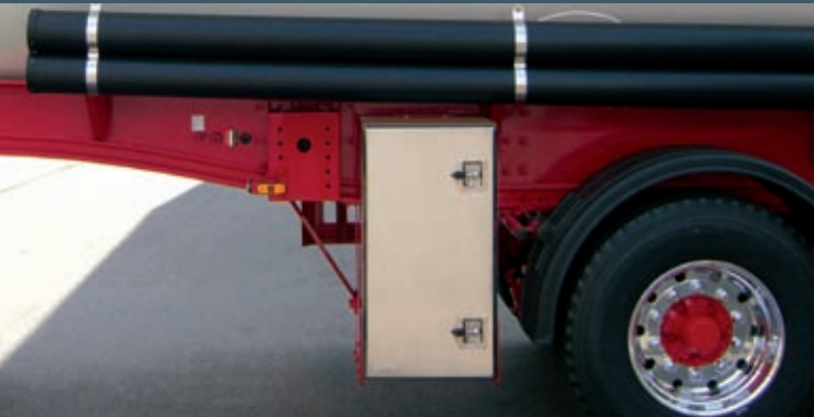
Semi trailer equipped with BAWER 36 DUO toolbox with lateral opening.
