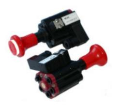
The Electrical Release (SP) The SP valves require an electrical signal to the integral solenoid valve before the valve may be operate and are ideal for interlocking with hand-brake electrical circuits for additional safety..
